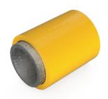
4mm (4,000 microns) thick PVC sleeved over galvanised steel tube after fabrication, giving 42mm or 50mm finished diameter. The double protection of galvanised tube and thick PVC sleeving is robust, will not chip and resists knocks and bumps.
